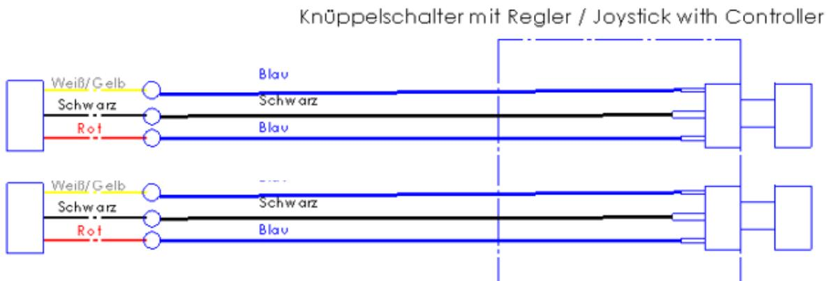
Use the 2-wire stick button instead of the built-in button SF left or SH right.
