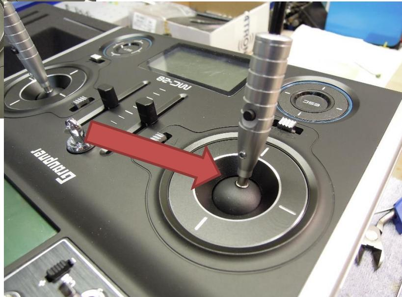
The buttons on the stick can be used in place of the existing ground button of the system. For this it is necessary to cut the wiring and to be soldered to the two shorter connecting wires of the stick.
