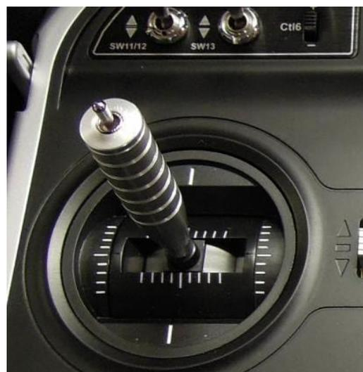
On older systems such as **MC 16, MC 19, MC 22 MC 24** recordings of the stick can be tighter. Some of the transmitter have only 3 mm holes. Here it is recommended to drill out the plastic holder with a 3.7mm drill at low speed and then wiped with a 3.8mm drill bit by hand.
